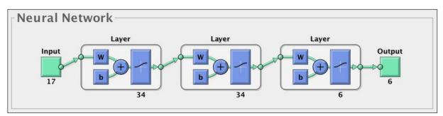
Fig. 4. The example of structure of used ANN
